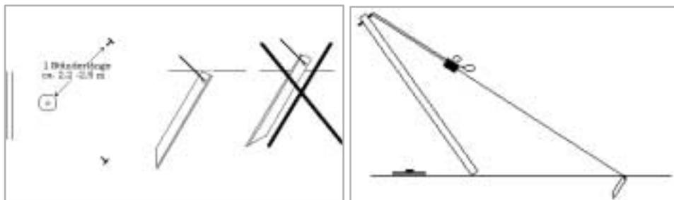
4. Place the posts next to the base plate. Hammer the pegs approx. one post section length from the base disc and roughly as shown into the ground. Hammer the pegs completely into the ground to prevent injuries from protruding parts. Only completely sunk pegs guarantee optimum anchoring.
