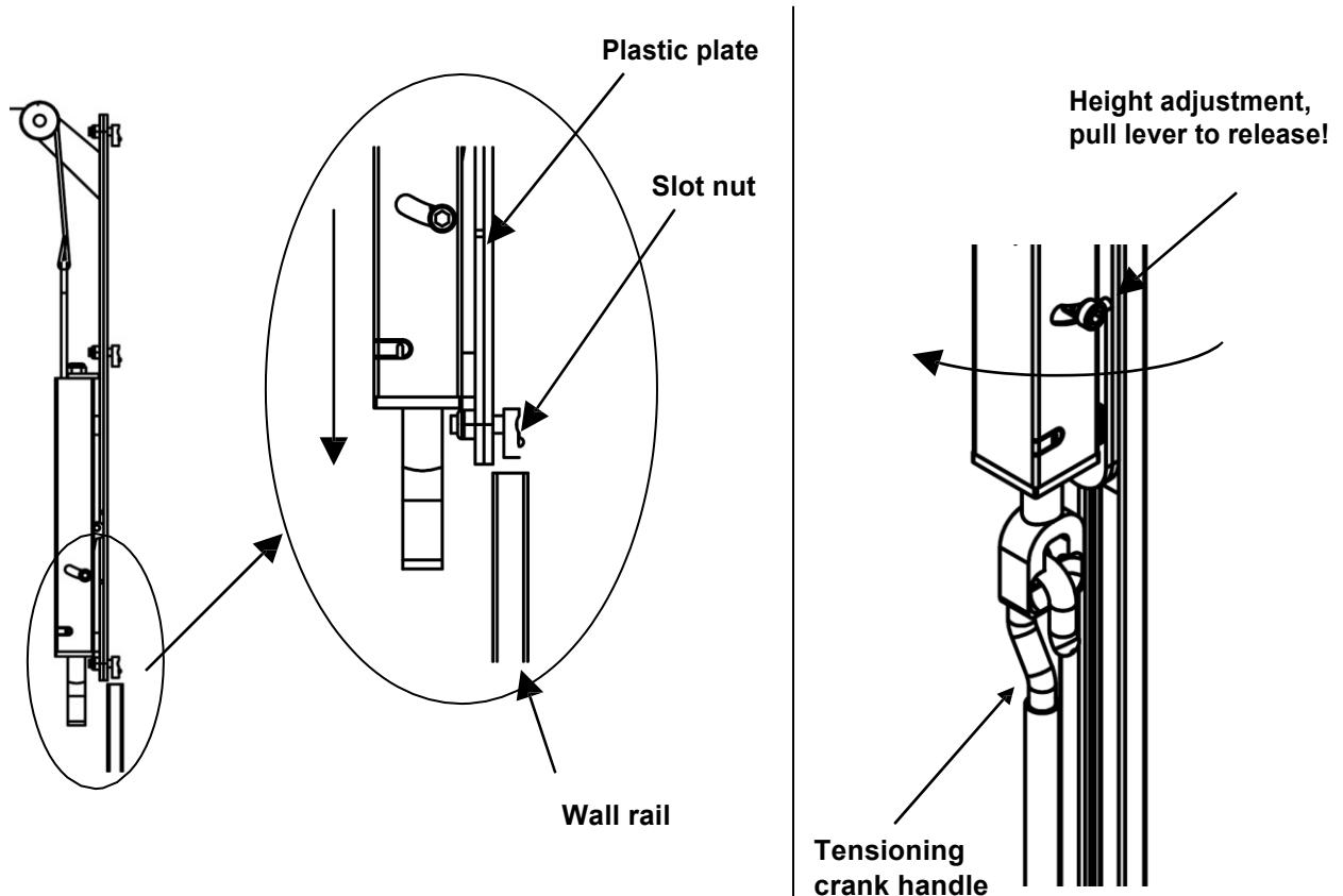
**III. 4: Mounting the tensioning device to the wall rail**
