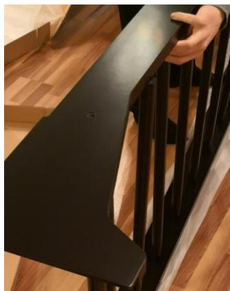
Fit the second rail on the top of the oval bars. Start at one end and progressively insert oval bars until all are seated. Use wooden block and rubber mallet if necessary to fully seat oval bars. Be careful not to damage or scratch the surface. Screw three oval bars to the
